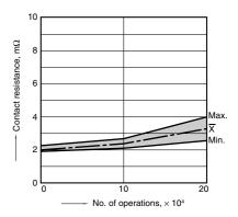
7-(2). Electrical life test (Lamp load)
